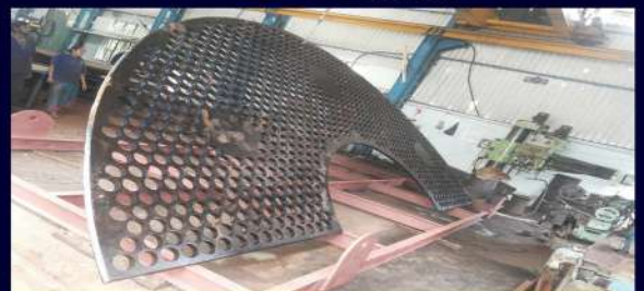
100 TON VACUUM PAN TUBE SHEET WITH S.S 410 MATERIAL. (EXPORTED TO VIETNAM)
