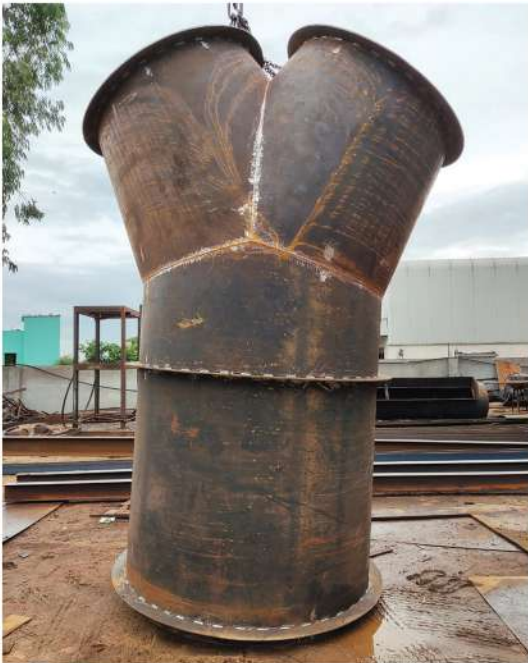
Y CONNECTION FOR DUCTING
